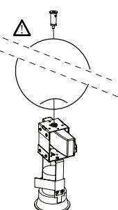
⚠ PULL GLOBE FOAM THROUGH WIRING
