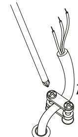
⚠ TIGHTEN UP THE STRAIN RELIEF AFTERWARDS.
