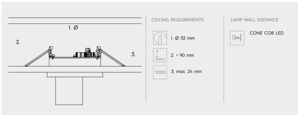
**1** Shut down power before installation
